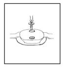
To change the stops, completely remove both screws from the hinge. Next, slide the hinge cover off.
